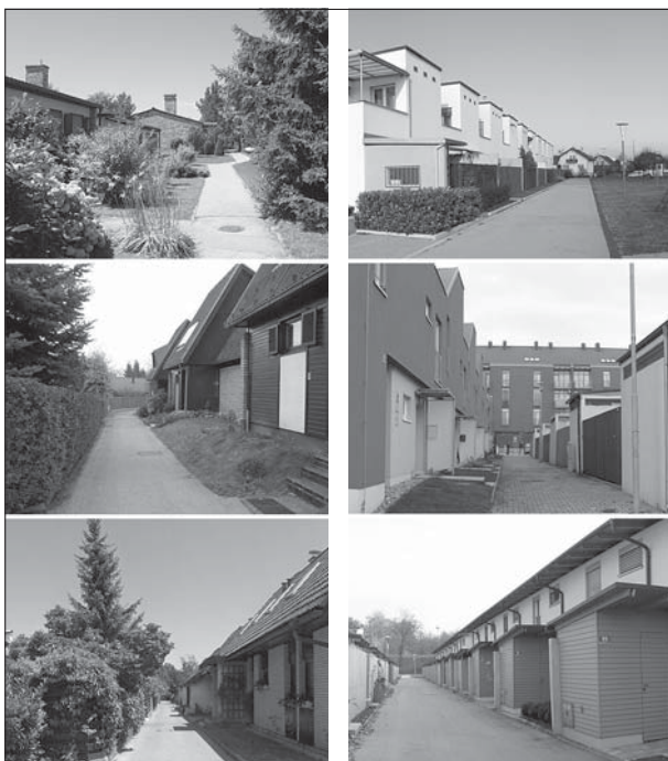
Figure 8: Street space and footpaths. In older settlements, footpaths were a part of the overall landscaping of the space (see examples on the left). New solutions decrease the size of these paths to a minimum (see examples on the right). (Photos: Nika Cigoj)
